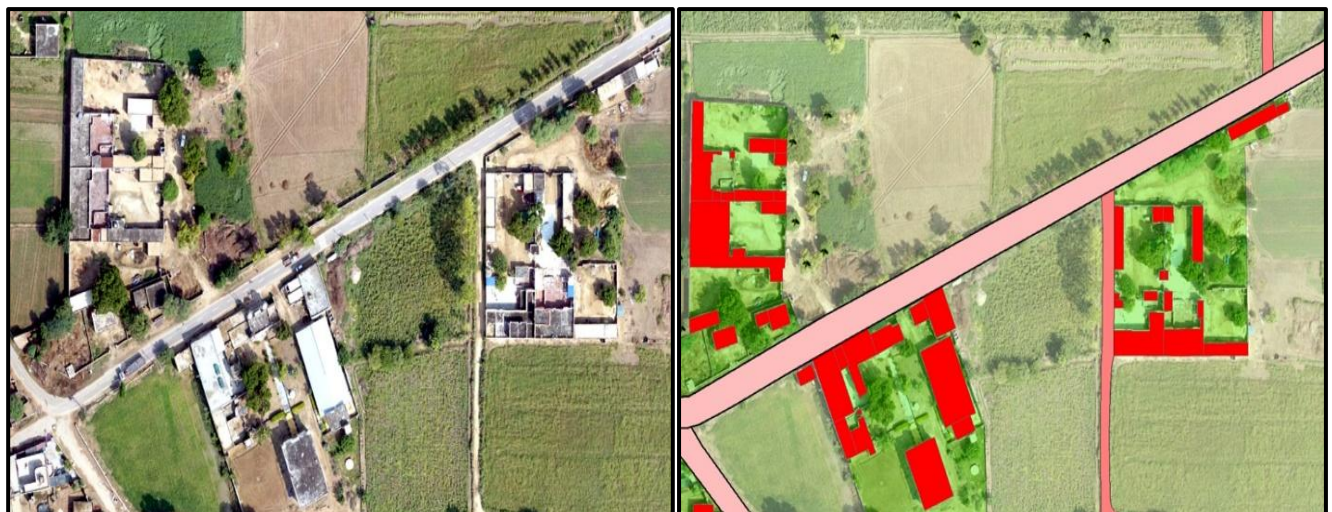
Fig 7: Ortho Rectified Image and feature extraction
