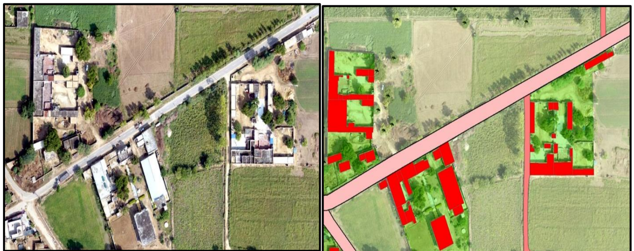
Fig 7: Ortho Rectified Image and feature extraction
