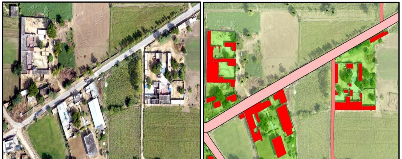
Fig 7: Ortho Rectified Image and feature extraction
