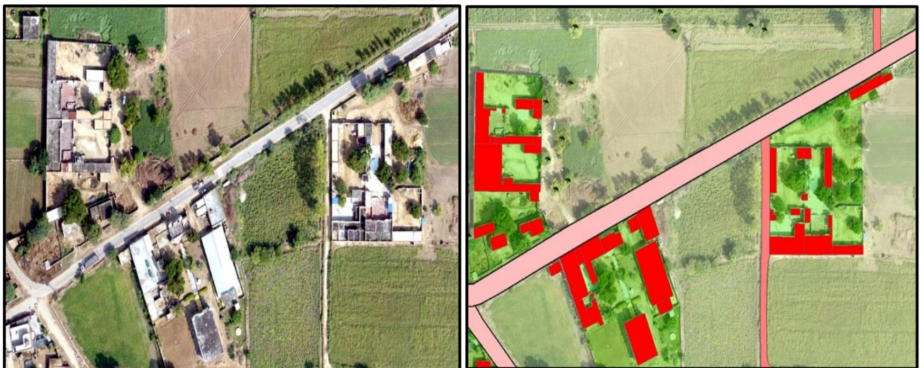
Fig 7: Ortho Rectified Image and feature extraction
