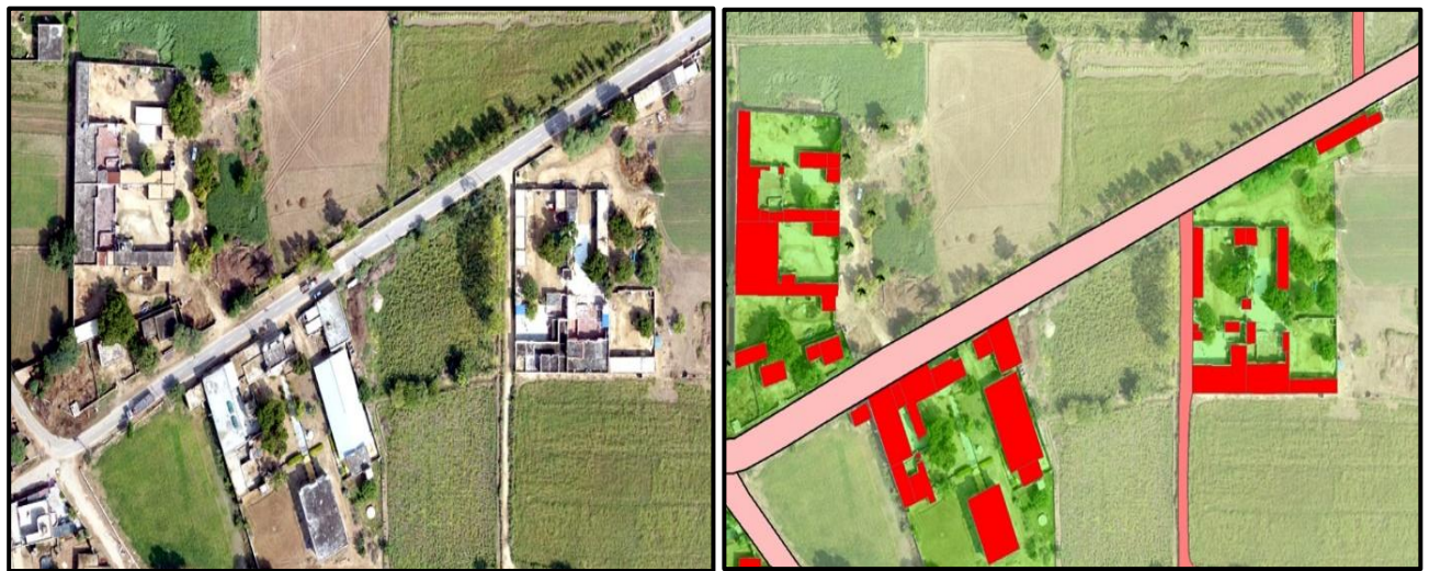
Fig 7: Ortho Rectified Image and feature extraction
