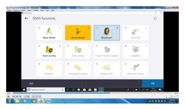
Step 11: Select paired Trimble R8s Rover receiver, which is just paired, for first two drop down menus as shown below and click Accept tab. Press Esc tab to return to main menu.
