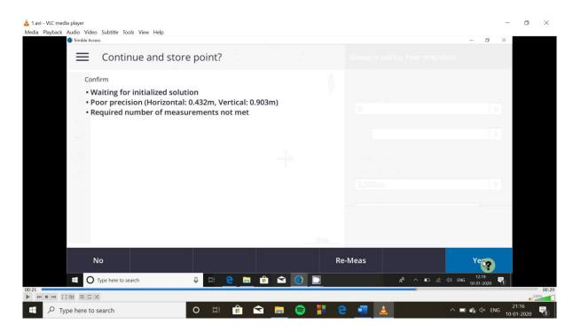
The Rover point collected will instantly give corrected coordinates with respect to Base.
