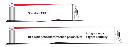
The aim of network RTK is to minimize the influence of the distance dependant errors on the computed position of a rover within the bounds of the network.
