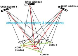
This correction information is then broadcast to users over web. The correction information depends on the processing algorithm and may include any of the following:
